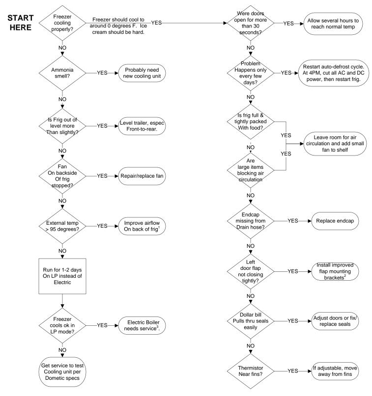
1. Add ventilator fan kit 3108705.744 (or equivalent) and check that baffle is directing air across the condenser fins before exiting top vent.
